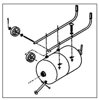
Figure 1. Wheel and handle installation.
